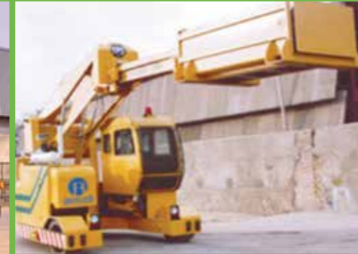
Furnace Charging Car
