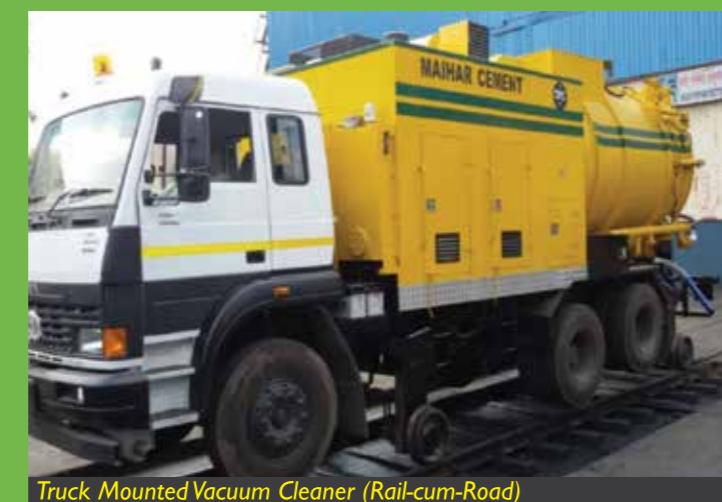
Truck Mounted Vacuum Cleaner (Rail-cum-Road)
