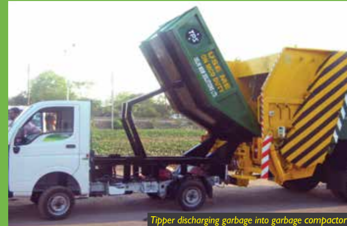
Tipper discharging garbage into garbage compactor
