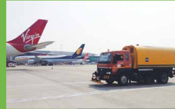
Truck mounted Road Sweeping Machine
