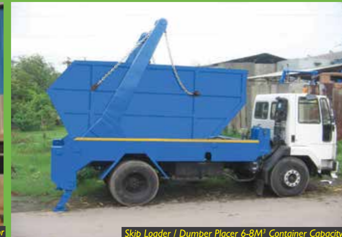
Skip Loader / Dumper Placer 6-8M³ Container Capacity
