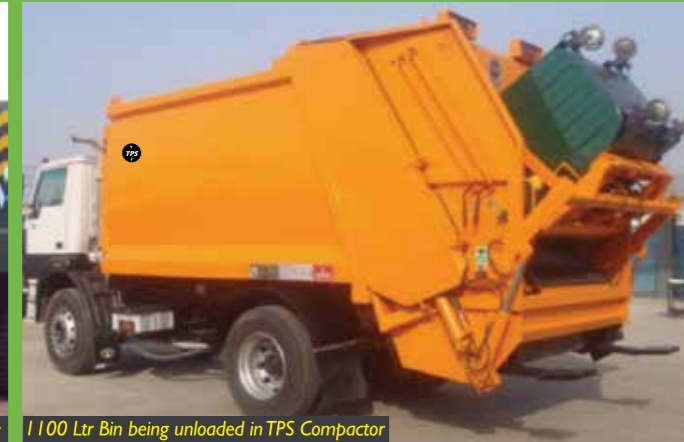
1100 Ltr Bin being unloaded in TPS Compactor
