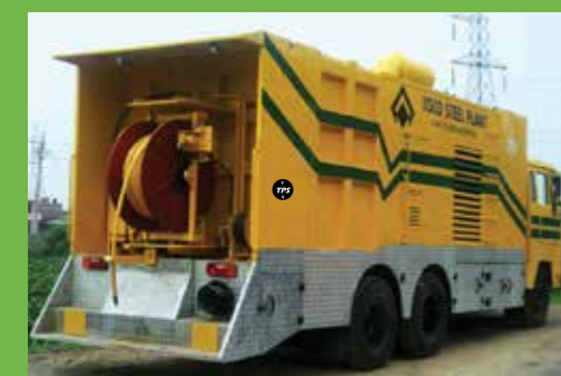
Desilting Machine for Cleaning of Trunk Sewer Pipelines
