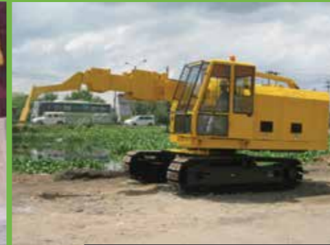
Furnace Tending & De-bricking Machine
