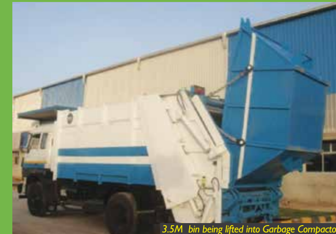
3.5M bin being lifted into Garbage Compactor
