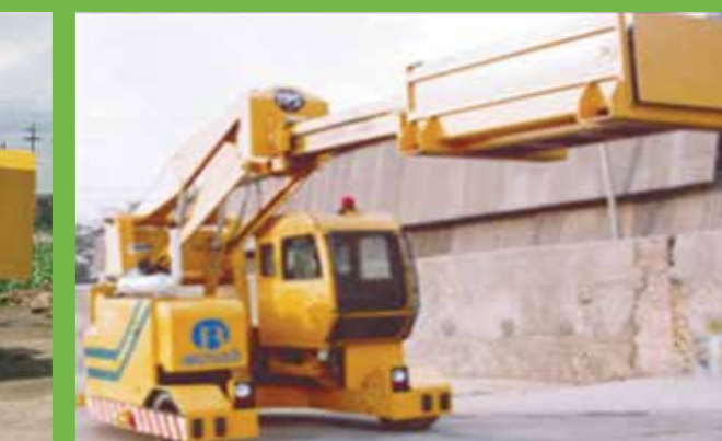
FURNACE CHARGING CAR
