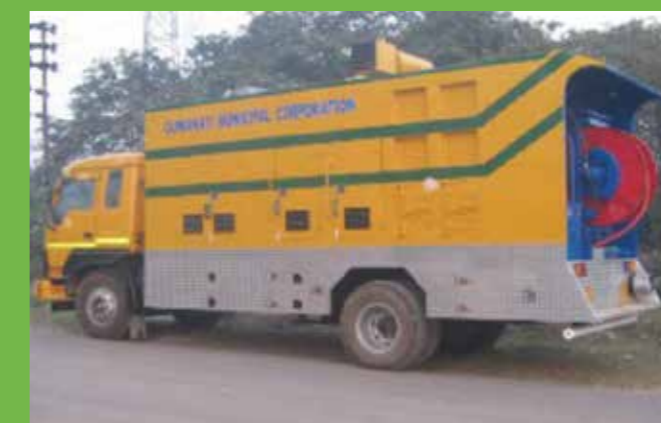
Super Sucker Vactruck Desilting Machine
