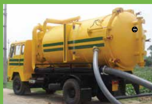
Suction Dump Tank with cyclone for collection of suctioned silt.
